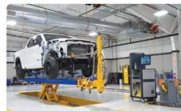
A Car-O-Liner machine at the Complex Repair Center in Baytown is set up to take measurements of the frame.
