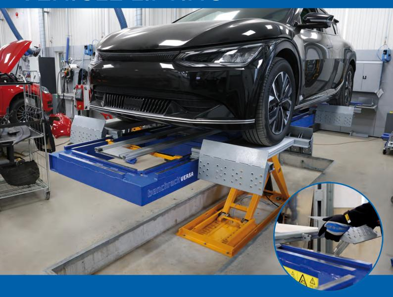
The new short ramps facilitate lifting by the wheels, allowing for a fast and secure process to position the vehicle at an optimal working height. The ramps are made of high-strength steel and aluminium to minimise weight and improve ergonomics.
